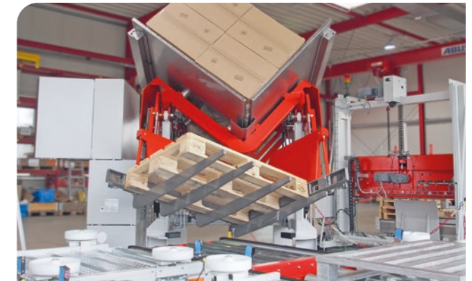
Innovative tilting pallet changer
