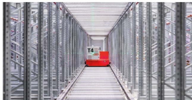
The fully automatic SMB compact storage systems: simultaneous storage and retrieval on every level
