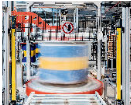
A stretch winder is also an integral part of the optimised filling process
